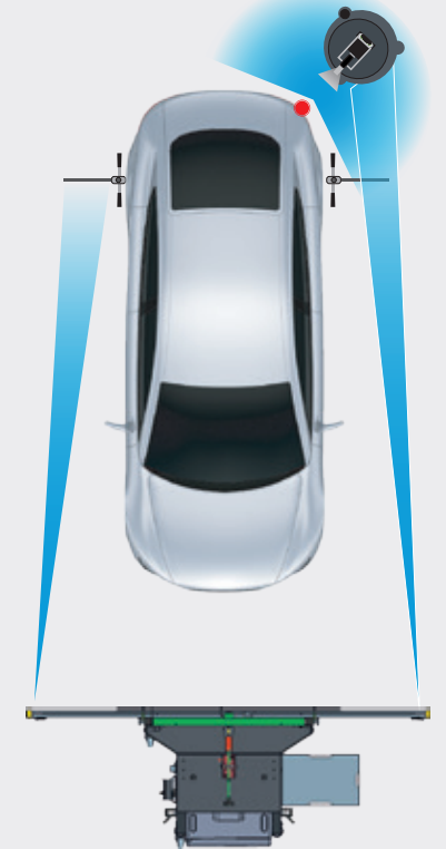
CTA 120 placement for corner radar with DAS 3000
