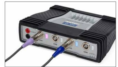
Colour guide in soft and hardware leads the user through automatic sensor recognition
