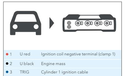
Detailed explanations and measurement descriptions help you when connecting the measuring adapter.
