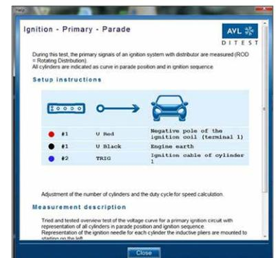
Assistance for connecting the measurement adapter via detailed explanations and measurement descriptions
