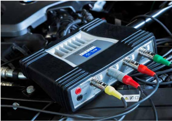
› 'Making the invisible visible' – visual representation of physical values such as voltage, power and pressure makes it easier to see complex interconnections when diagnosing faults
