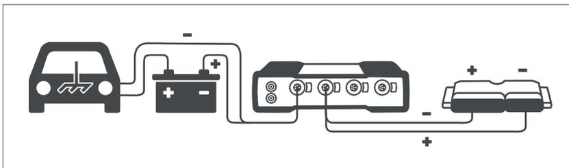
Easily measure voltages from various sources with reversed polarity.
